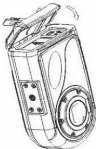
10. Press and hold the battery door down as shown in diagram (a). Gently lift the lever (2) upwards until you hear it click and lock into place as in diagram (b). Now push the middle section of the battery door to the left as indicated in diagram (c).
