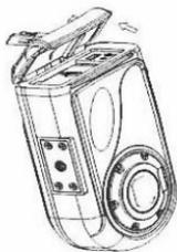
5. In order to open the battery compartment, locate the OPEN arrow pointing down on the battery compartment door and press down in the direction of the arrow.
